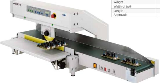
For separating aluminum with the MAESTRO 4S the standard circular blade with special blade settings can be used. More information in the operation manual and at **www.cab.de/en**
