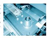
Highest process reliability is ensured with an automatic solder wave monitoring and wave height control as well as a solder level control.
