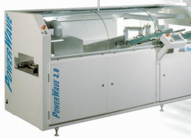
The Chip wave promotes wetting in critical areas of the assembly because of its high kinetic energy. The Delta wave offers long immersion times and excellent surface definition and thus forms optimal solder joints.
