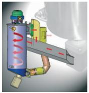
A new feature is that <u>all</u> of the heated zones are directly connected to the system for cleaning the process gas. Moreover, the removed process gas is conducted within the hot area up to the cleaning point, in order to guarantee that the condensation is controlled. The cleaning system itself is the first cold point
