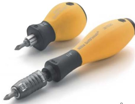
The Wiha SoftFinish® ESD with integrated soft zone is eminently suitable for working with electrostatically endangered construction components in ESD protected zones. The dissipative handles with a surface resistance of 106 - 109 ohms conduct electrostatic energy away from endangered electronic components in a controlled and safe way.
